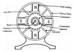
All electrical machines have mainly two parts-Stator (stationary part) and Rotor (rotating part)
